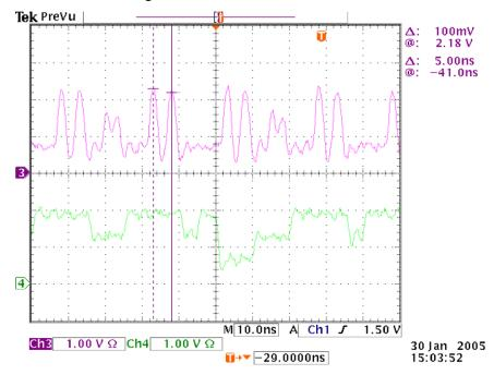
Figure 10-23. WRITE to READ Transition Running at 200MHz
