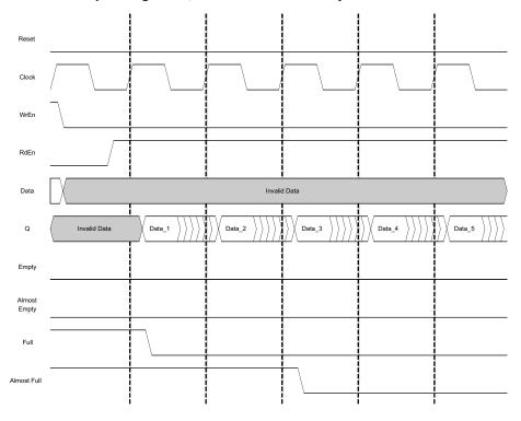
Figure 9-35. FIFO Without Output Registers, Start of Data Read Cycle
