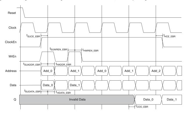
Figure 9-10. Single Port RAM Timing Waveform - NORMAL Mode, with Output Registers
