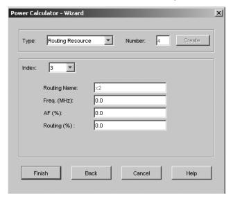
Figure 12-12. Power Calculator Wizard Mode Window - Resource Specification - I/Os
