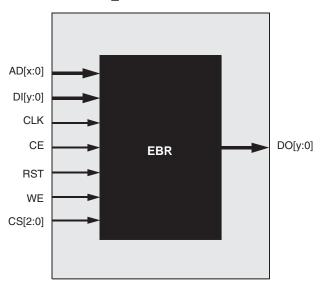
In Single Port RAM mode the input data and address for the ports are registered at the input of the memory array. The output data of the memory is optionally registered.
