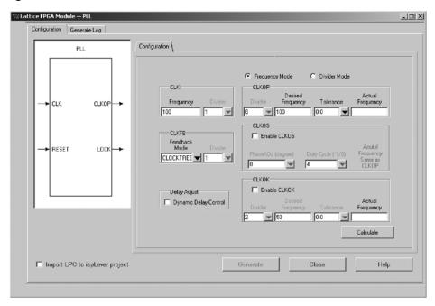
**Divider Mode**: In this mode, the user sets the input frequency and divider settings. It is assumed the user is familiar with the PLL operation. The user must choose the CLKOP Divider value to maximize the f<sub>VCO</sub> to achieve optimum PLL performance. After input frequency and divider settings are set, clicking the 'Calculate' button will display the output frequencies. If the divider settings are out of the PLL specification, the software will generate an error.
