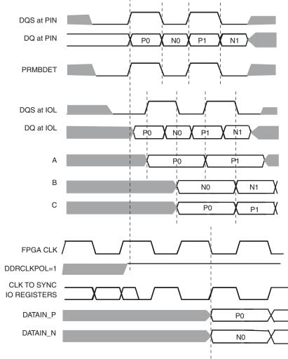
Figure 10-13. Read Data Transfer When DDRCLKPOL=1
