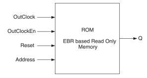
The generated module makes use of these EBR blocks or primitives. For memory sizes smaller than an EBR block, the module will be created in one EBR block. If the specified memory is larger than one EBR block, multiple EBR blocks can be cascaded, in depth or width (as required to create these sizes).
