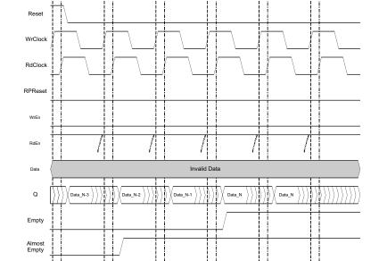
Figure 9-45. FIFO\_DC Without Output Registers, End of Data Read Cycle
