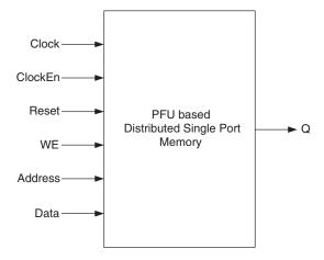
The generated module makes use of the 4-input LUT available in the PFU. Additional logic like Clock, ClockEn and Reset is generated by utilizing the resources available in the PFU. The basic Distributed Single Port RAM primitive for the LatticeECP/EC and LatticeXP devices is shown in Figure 9-52.
