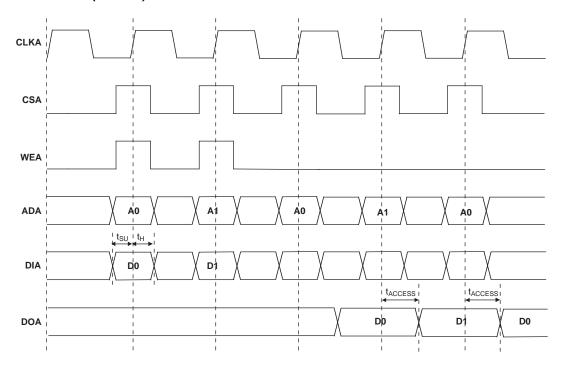
Note: Input data and address are registered at the positive edge of the clock and output data appears after the positive of the clock.
