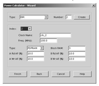
Figure 12-10. Power Calculator Wizard Mode Window - Resource Specification - PLL
