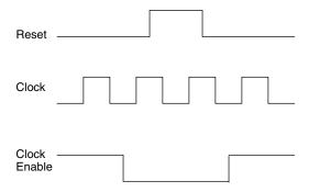
If all clock enables remain enabled, the EBR asynchronous reset or GSR may only be applied and released after the EBR read and write clock inputs are in a steady state condition for a minimum of 1/f<sub>MAX</sub> (EBR clock). The reset release must adhere to the EBR synchronous reset setup time before the next active read or write clock edge.
