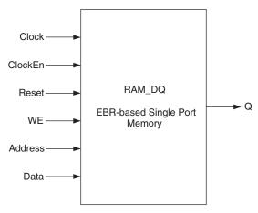
Since the device has a number of EBR blocks, the generated module makes use of these EBR blocks or primitives and cascades them to create the memory sizes specified by the user in the IPexpress GUI. For memory sizes smaller than an EBR block, the module will be created in one EBR block. In cases where the specified memory is larger than one EBR block, multiple EBR block can be cascaded, in depth or width (as required to create these sizes).
