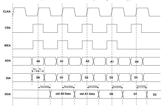
Figure 3-10. Read Before Write (SP Read/Write on Port A, Input Registers Only)
