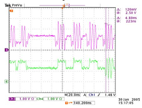
Note: An extra READ command is implemented in the LatticeEC20 device to protect the data during postamble. This extra READ is not required for other LatticeEC devices. Refer to the DQS Postamble section of this document for more information.
