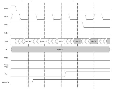
Figure 9-34. FIFO Without Output Registers, End of Data Write Cycle
