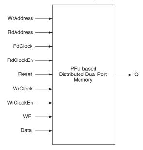
The generated module makes use of a 4-input LUT available in the PFU. Additional logic for Clocks, Clock Enables and Reset is generated by utilizing the resources available in the PFU. The basic Distributed Dual Port RAM primitive for the LatticeECP/EC and LatticeXP devices is shown in Figure 9-56.
