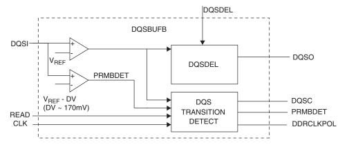
Figure 10-7 shows the primitive symbol and its ports. DQSI is the DQS signal from the memory. PRMBDET is the preamble detect signal that is generated from the DQSI input. READ and CLK are user interface signals coming from the FPGA logic. The DQSDLL block sends digital control line DQSDEL to this block. The DQS is delayed based on this input from the DQSDLL. DQSO is the delayed DQS and is connected to the clock input of the first set of DDR registers.
