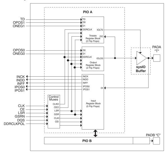
In the LatticeXP family, seven PIOs or four (3.5) PICs are grouped together to provide two LVDS differential pairs, one PIC pair and one single I/O, as shown in Figure 2-18.
