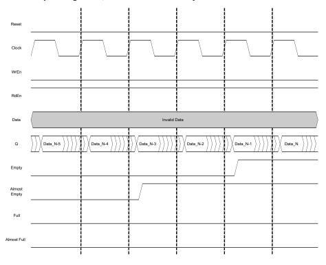
Figure 9-40. FIFO with Output Registers, End of Data Read Cycle
