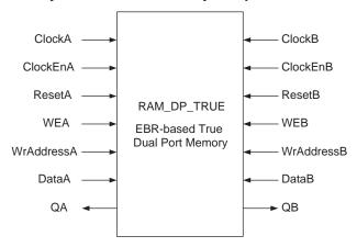
The generated module makes use of the RAM\_DP\_TRUE primitive. For memory sizes smaller than one EBR block, the module will be created in one EBR block. In cases where the specified memory is larger than one EBR block, multiple EBR blocks can be cascaded, in depth or width (as required to create these sizes).
