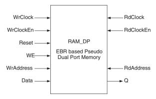
The generated module makes use of these EBR blocks or primitives. For memory sizes smaller than an EBR block, the module will be created in one EBR block. If the specified memory is larger than one EBR block, multiple EBR block can be cascaded, in depth or width (as required to create these sizes).
