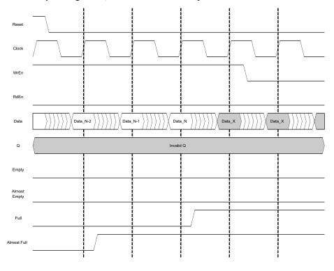
Figure 9-39. FIFO with Output Registers, Start of Data Read Cycle
