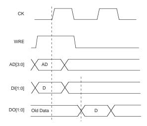
Figure 3-7. Slice Single /Dual Port Read Cycle Timing
