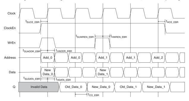
Reset Clock t<sub>SUCE\_EBR</sub> t<sub>HCE\_EBR</sub> ClockEn tsuwren\_ebr t<sub>HWREN\_EBR</sub> WrEn t<sub>HADDR\_EBR</sub> t<sub>SUADDR\_EBR</sub> Add\_0 Add\_0 Add\_1 Address Add\_1 Add\_2 New New Data Data\_0 Data\_1 t<sub>SUDATA\_EBR</sub> thdata ebr New Q Invalid Data Old\_Data\_0 New\_Data\_0 Old\_Data\_1 Data\_1 t<sub>COO\_EBR</sub>
