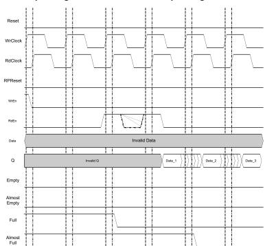
Figure 9-50. FIFO\_DC With Output Registers and RdEn on Output Registers
