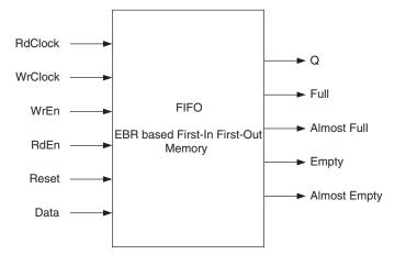
LatticeECP/EC and LatticeXP devices do not have a built in FIFO. These devices have an emulated FIFO and FIFO\_DC. These are emulated by creating a wrapper around the existing RAMs (like RAM\_DP). This wrapper also includes address pointer generation and FIFO flag generation logic which will be implemented external to the EBR block. Therefore, in addition to the regular EBR usage, there is extra logic for the address pointer generation and FIFO flag generation.
