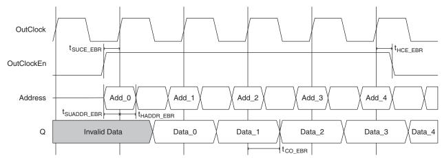
Figure 9-30. ROM Timing Waveform - with Output Registers
